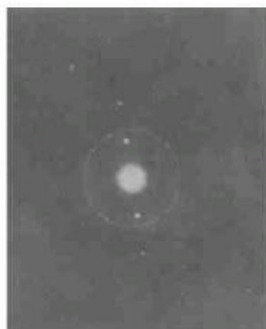
Fig.6 Electron diffraction photograph of C*PPO/PS blends. Annealing temperature: 240 °C Annealing time: 20 min
